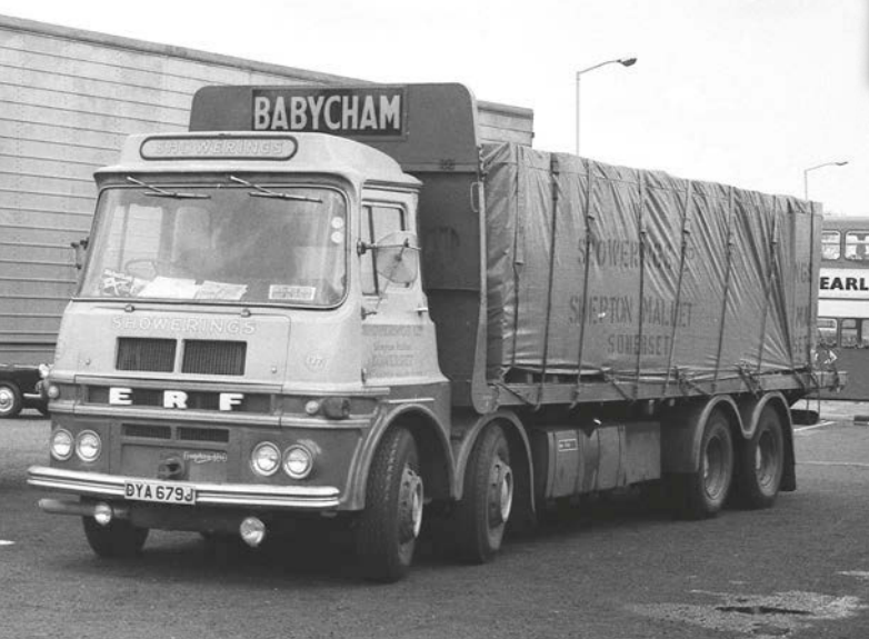
Above: ERF LV-cabbed 68G – Gardner-powered eight-wheeler, DYA 679J (Somerset, 1971), of Showerings of Shepton Mallet, with the customary tall headboard carrying the 'Babycham' name, seen at Keele Services on the M6 in 1974, with a full load of the bubbly stuff, and later with a frame body, loaded with the dodgems track, believed to be in the fleet of Anderton & Rowland.
