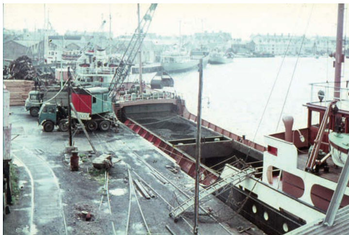
Above: The Smiths of Rodley mobile crane, fitted with a grab by the operator, Jim Thorpe of Paignton, mounted on a Foden DG eight-wheeler, unloading coal from a ship's hold, into an LAD-cabbed Dodge tipper of W L Vallance in July 1967.
