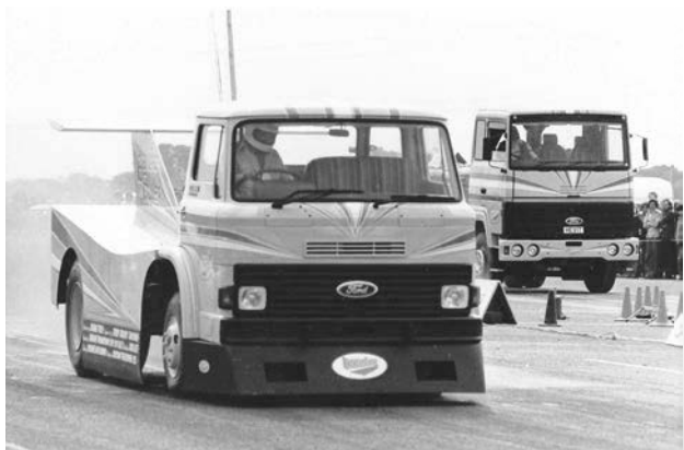
Above: All work and no play makes D a dull boy. The 'Bandag Bullet', which promoted the company's re-treaded truck tyres, was a souped-up D1314 tipper chassis, with 300 hp replacing the standard 140 hp, giving it a top speed of 108 mph! (Richard Stanier)
