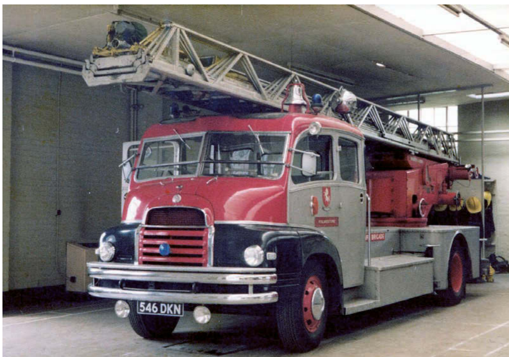
Above: This elaborate-looking turntable ladder was one of four in service with Kent Fire Brigade. Delivered in 1958, it was pictured at Folkestone fire station in 1976. John Morris & Sons Ltd, of Salford, was the import agent for the German Magirus ladder, the coachwork being sub-contracted to Wilsdons of Solihull.
