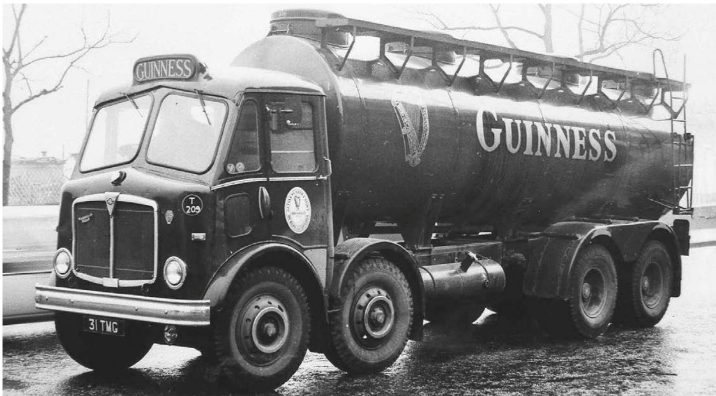
Above and right: This 'Tin front' AEC Mammoth Major Mk III, 31 TMG (Middlesex, early 1959), is seen working as a tanker in the Guinness fleet, based at Park Royal, and 'on the tober', probably around 20 years later, fitted with a sheeted frame truck body, working for London area amusements caterer, John Biddall.
