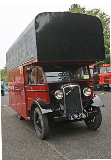
Above: Getting the Wind-up? The huge 'Luton' head on this 1934 Commer 'Raider' van must have been handful on a windy day – especially when empty! The bodywork was built by original operator, Burns & Symonds, based in South London. It was requisitioned during the war and used as transport for Air Raid Wardens.
