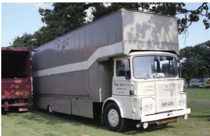
Above and below: This Guy Big J four-wheeler, HHP 401N (Coventry, 1974), underwent quite a change of bodywork, from a car transporter for the Toleman Group, to a Luton box van for Ron Taylor's Amusements.
