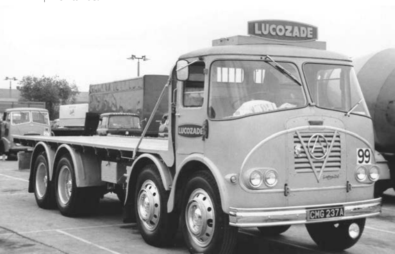
Above: A fleet from which many lorries went on to be used by showmen was that of Lucozade, whose Garder-powered Atkinson eight-wheeler, fitted with the short-lived front panel, concealing the radiator, CMG 237A (Middlesex, 1963), is seen when quite new at an LDOY heat, and again, later in life, with a frame truck body, working for a showman.
