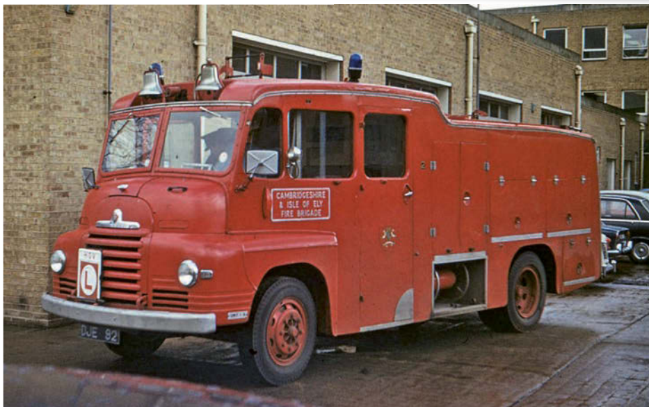
Above: This unusual machine was one of three water tenders delivered to Cambridge and Isle of Ely Fire Brigade in 1953. Cuerdon Motor Bodies of Blackburn built the bodywork. This firm built many fire engines on Commer chassis, but the only Bedfords were these ones for Cambridgeshire.
