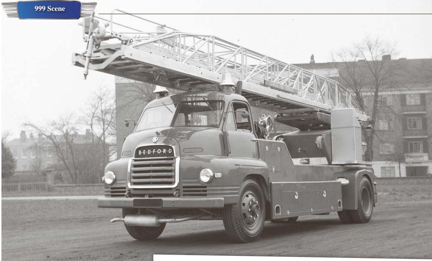
Above: The Bedford S was sold to overseas customers for a multitude of applications and fire engines were no exception. This turntable ladder with two man cab and 100 ft Merryweather ladder was exported to Cyprus and is still in existence on the island.
