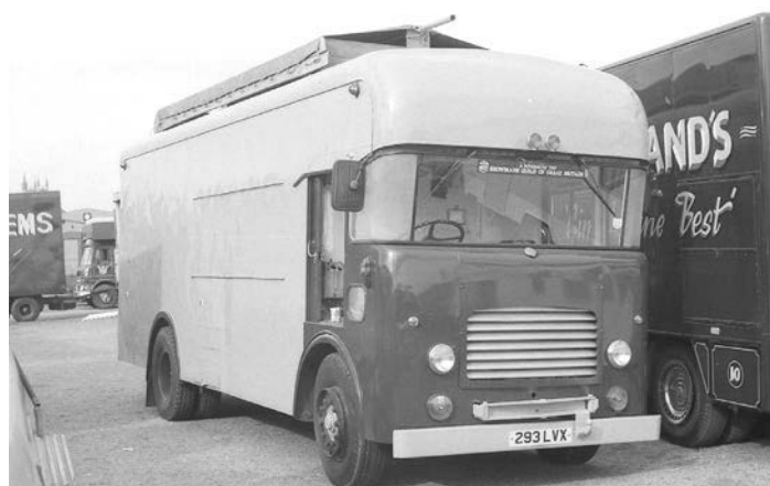
Above and below: With its unusual integral van bodywork, this Leyland, presumably with a Comet chassis, 293 LVX (Essex, 1958), was working for Smiths, the auto-electrical company, when it was photographed at an LDOY heat, before being used by showman, G Floyd Junior, with a canvas-covered rack added to its roof.
