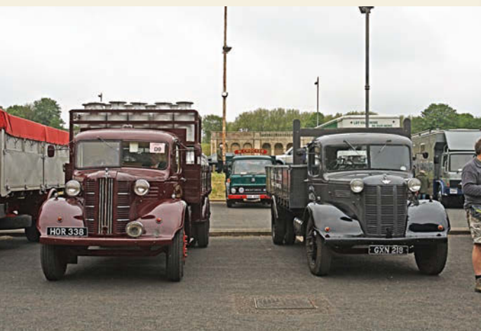
Above: Seeing Double. On the left is HOR 338, the post-war Austin K4 dropsider with the milk churn load. And on the right is GXN 218, a pre-war model. Note the different radiator grille design.
