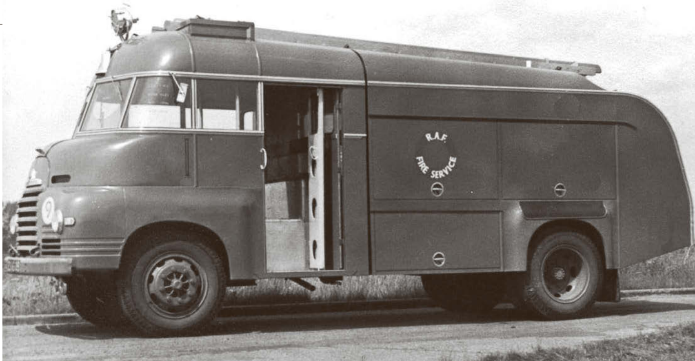
Above: The Royal Air Force's 'Domestic tender' had the profile of the Alfred Miles standard water tender, but the Ministry of Supply's specification required several amendments such as different locker covers, full height doors, roof hatch and larger water tanks.
