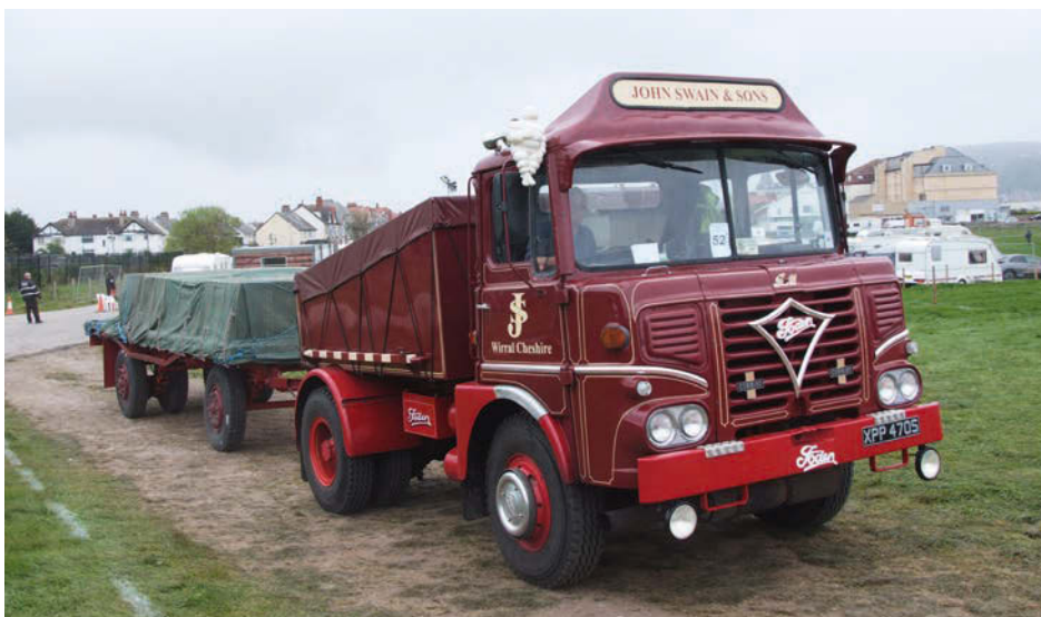
Above: A Cummins-powered Foden ballast tractor, with the S41 cab, XPP 470S (Buckinghamshire, 1978), in the livery of John Swain & Sons, from the Wirral, pulls onto Bodafon Fields, with a suitable trailer, complete with four-in-line split rear axles. (VC)
