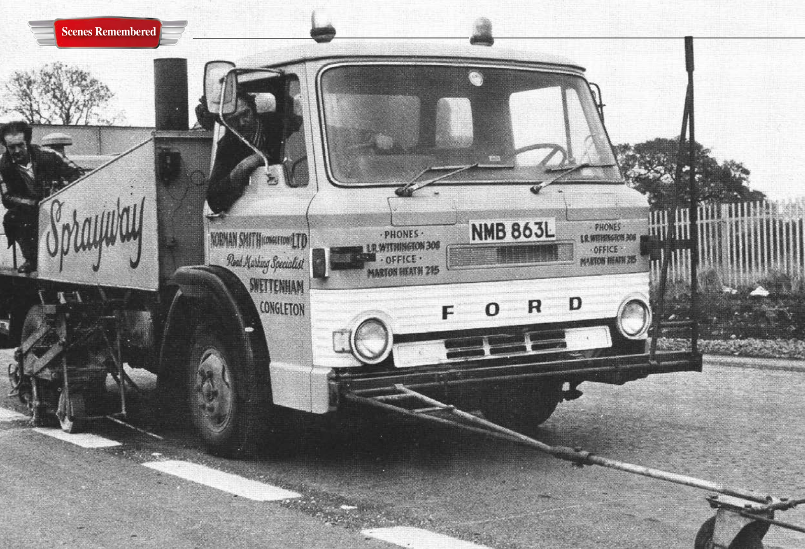
Above: The D Series could turn its hand to anything and this wagon was designed specifically for painting road markings. This short wheelbase, 4-tonner was a special build, with low gear ratios and both left and right hand steering.
