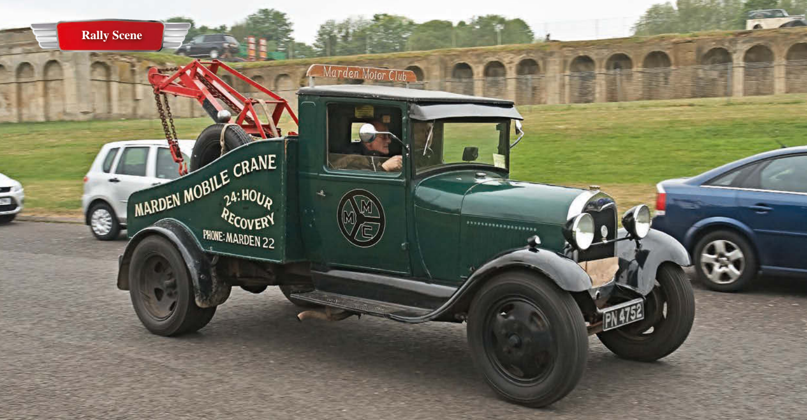
Above: Heading for a breakdown? This Ford Model AA was donated to the Marden Motor Club in the 1960s and has retained a wonderful well-used look ever since. It still runs the original 24 hp engine, which has recently been rebuilt.
