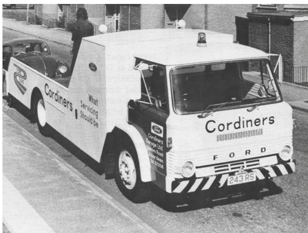
Above: What better way of showing commitment to the brand than operating a D Series breakdown wagon. Ford Dealer, Cordiners of Aberdeen did just that in the mid to late 1960s and operated this 4-tonner, with an interesting style of partially-enclosed beaver-tail bodywork. Notice that the car being recovered is not a Ford...
