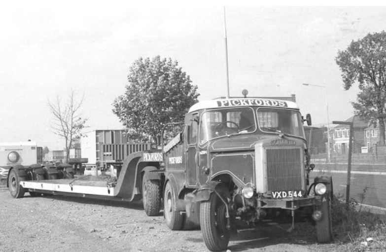
Above: Scammell Highwayman ballast tractor, VXD 544 (London, 1958-59), M2084 in the Pickfords fleet is seen with a draw-bar low-loader trailer, with four-in-line bogies, awaiting its next load, and as 'Happy Wanderer', with amusements operator, Roberts & Son, of Bourne End, Buckinghamshire, its usual ballast box body extended at the rear to accommodate the customary generating set.
