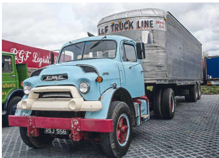
Above: The US-built 1954 Detroit 671 six cylinder two-stroke diesel-powered GMC model 863, with 1950 Freuhauf stainless steel-bodied trailer, lettered L&F Truck Line, Denver.
