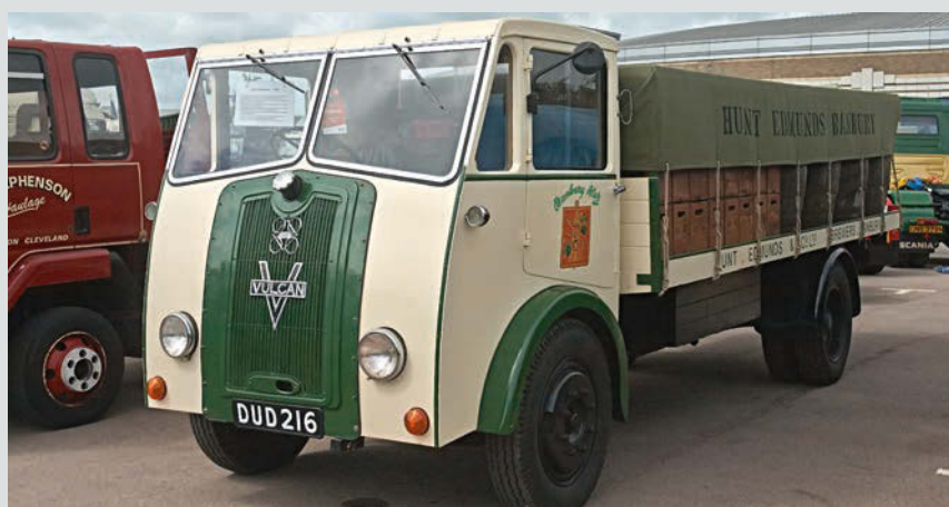
Above: A wagon with a story. This Vulcan (chassis number 3802) was supplied to Hunts Edmunds Brewery of Banbury in 1948, powered by a petrol engine. This was changed for a Perkins P6 in 1953 and it remained in service until the early 1960s, when it was 'retired' to be used on farm. Rescued by the Humphries family in 1990, it was finally put back on the road in 2012. Mr Humphries Senior even made a complete set of wooden crates to give a period-look load – based on a single surviving example!
