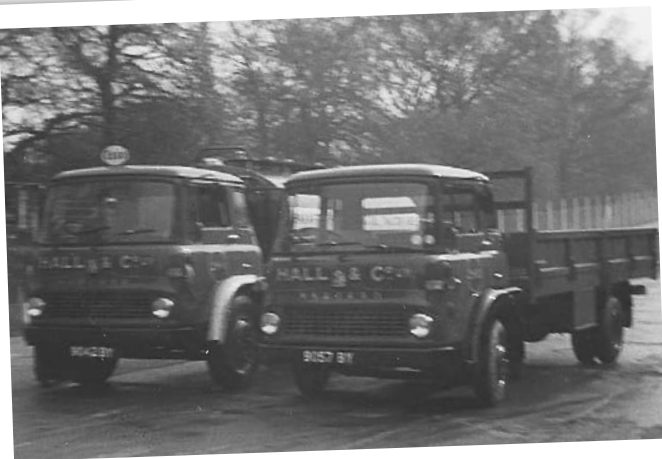
Above left: Hall & Co used the Bedford TK in its fleet for many different purposes as well as tipper chassis, like these two 1961 lorries, a 5 ton dropside, with the 16 inch six-stud wheels (what would later become a 7½ tons gross non-HGV), 9057 BY, and a 12-tonner, with 20 inch wheels, 9042 BY, bodied as a tanker, for the fuel oils side of the business. (Geoff Heels) Above right: Phil mentions the Bedford WTL dropside he was involved with restoring, along with the other apprentices, which is believed to have since passed to Vauxhall Motors' collection. Hall & Co also restored this 1934 AEC Matador, OY 9542, seen here on the London to HCVC Brighton Run in the late 1960s or early 1970s. After some time in the British Commercial Vehicle Museum in Leyland, it has more recently been seen in the livery of J Henslow & Sons of Macclesfield. (Stevens-Stratten Vintage Roadscene Picture Library)
