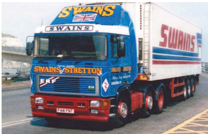
Above: There were also ERFs in the Swains fleet, like this E14 three-axle tractor unit, F441 FNT (Shrewsbury, 1988-89), seen with a tri-axle reefer – running on six axles was considered a good way to save a lot of road tax at the time – coming down the ramp off the A2 into Dover Docks.
